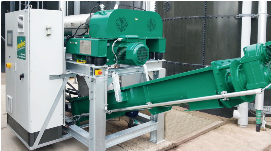
Mobile centrifuge dewatering unit with CT-350 decanter centrifuge - location Germany
