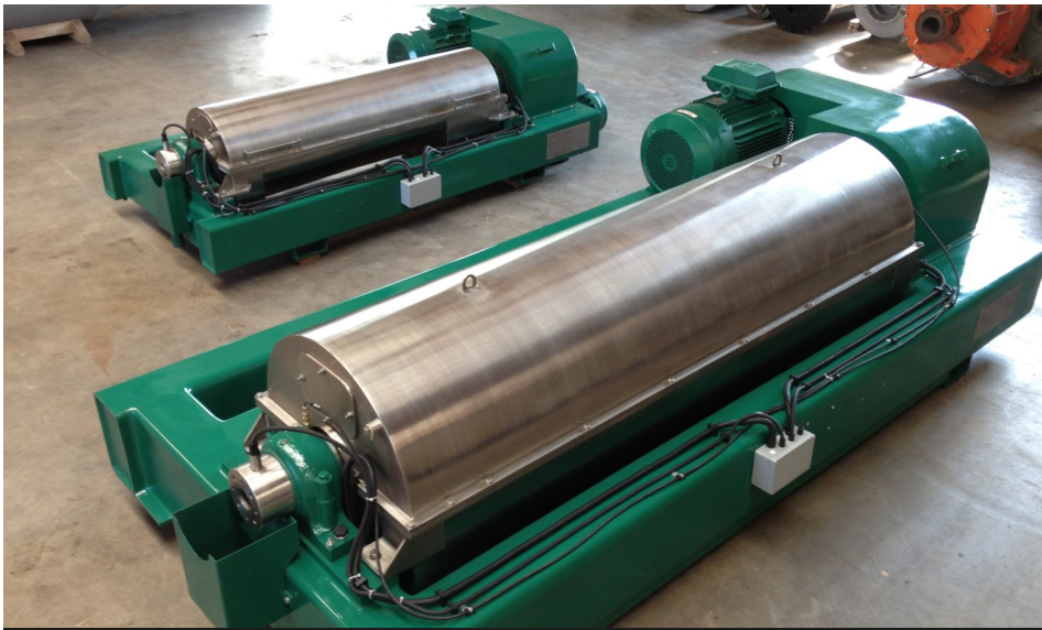
CT-530 and CT-350 with bearing temperature monitoring and automatic greasing system
