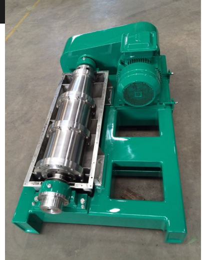
CT-530 and CT-350 with bearing temperature monitoring and automatic greasing system
